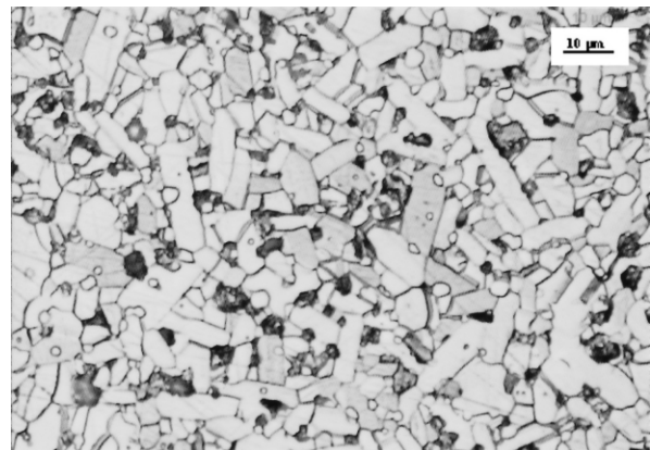
Fig. 2. Microstructure of BCSiC material (Murakami's etching).
